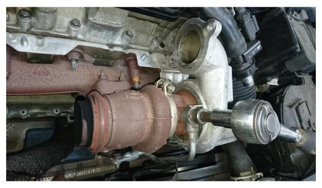
The next step is to loosen the 4 11mm nuts holding the turbo to the manifold. If these are tight you might want to join two spanners together to get some extra leverage.
