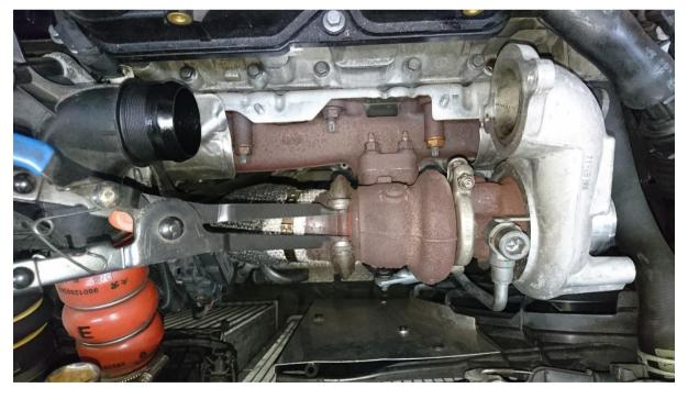
The exhaust clamp uses a 16mm nut at the bottom and then you can use a tool as shown above to remove the v band clamp.
