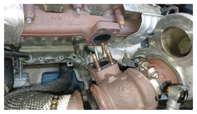
Before you refit the turbo, you will need the correct oil pipe (part number 63846), as shown here the pipe for the GTD1244VZ is completely different. I would also recommend fitting new banjo bolts. Don't remove the strainer from the lower bolt, it's a filter and an oil restrictor, removing it will cause future problems.
