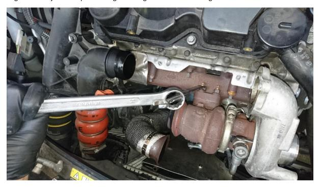
With the four nuts off you can slide the turbo outwards and then you'll be able to easily see the turbo oil drain. Loosen the 7mm nut on the jubilee clamp and then pop the hose off. The turbo will now come out.
