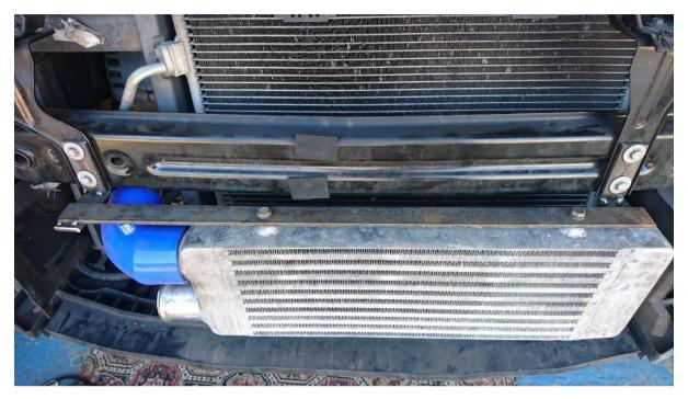
Once you're happy the bracket is the correct size and that the bumper will fit back on you can weld it fully and paint it to prevent rust.
