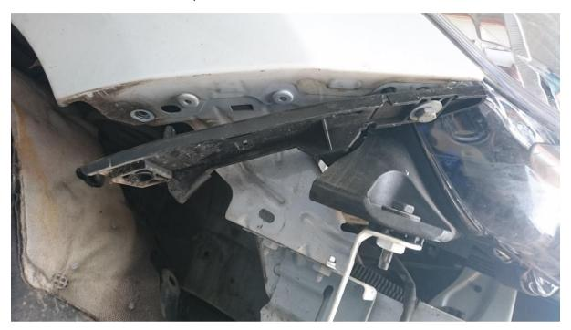
Once the bumper is off you can remove the front beam to give enough space to remove the stock intercooler. Here's a comparison of the stock intercooler versus the upgraded intercooler. The area is around double and it will be in a much better position behind the grill with much better air flow to keep it cool.
