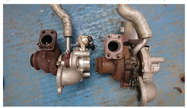
The position of the oil drain and the oil feed is the same, so it's quite an easy conversion.
