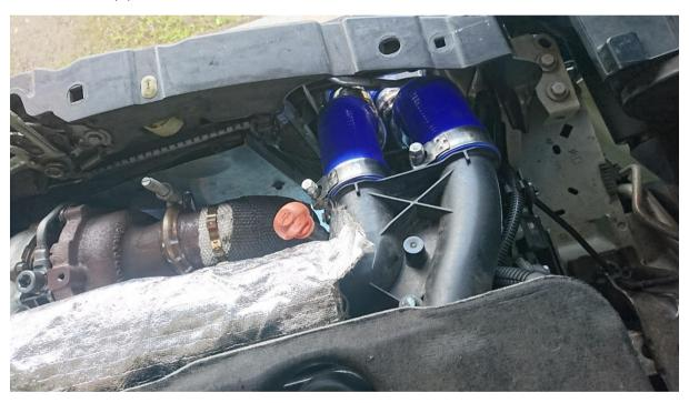
Here's the final job with the intercooler and pipe work fitted.
