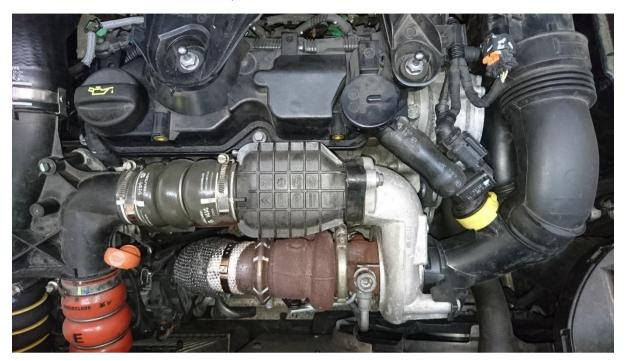
Remove the intake pipe which is held on with a 10mm bolt, and the turbo outlet to intercooler pipe which has two 10mm bolts and the jubilee clip uses a 7mm socket.
