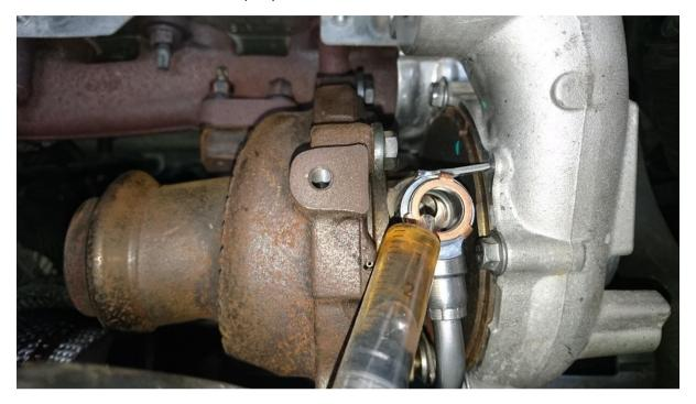
When you come to connect the plug to the turbo actuator position sensor you will find that it has been designed to prevent you from connecting it to the wrong turbo. To get the extra length on the wire you simply need to remove the 90-degree collar that is clipped on to the wire.
